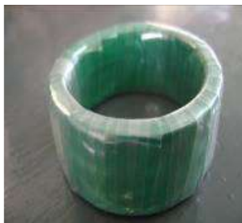
The finished taped core
