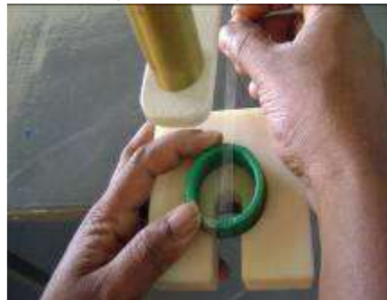
Hold tape over top of toroid
