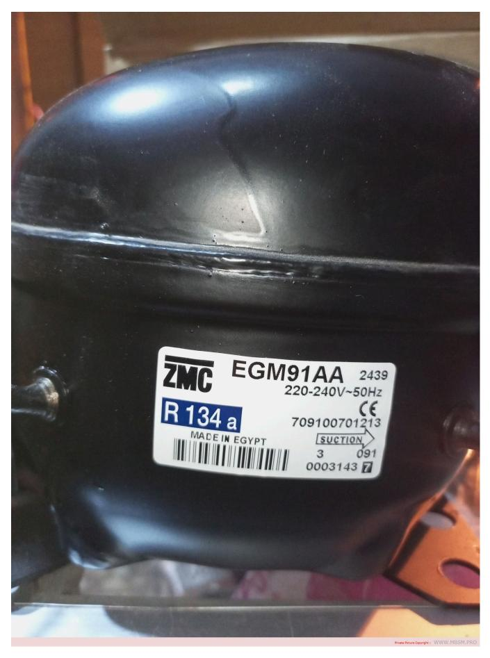
The EGM91AA compressor from ZMC stands out as one of the most notable solutions in the domestic and light commercial refrigeration sector thanks to its use of R134a refrigerant and its high efficiency under varying climatic conditions. It delivers optimal cooling performance for
