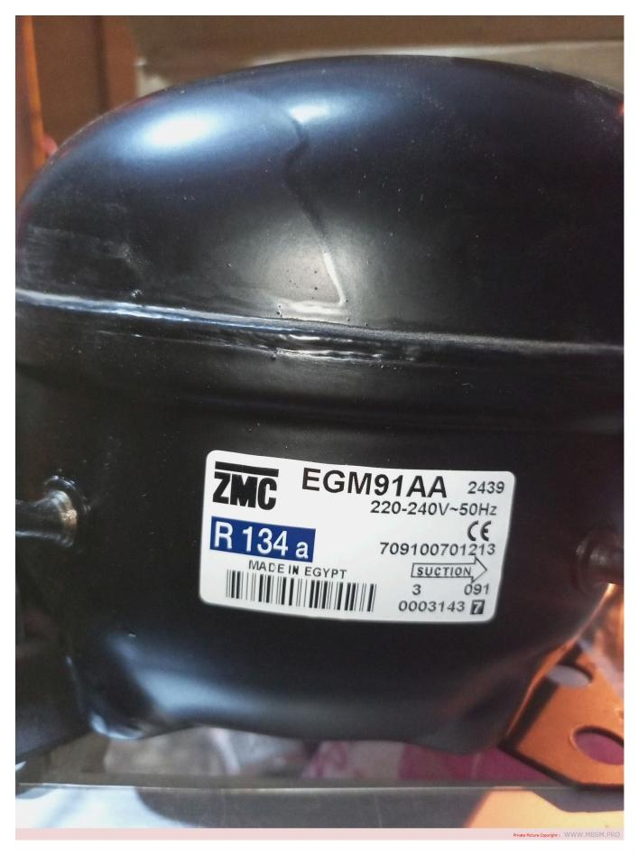
The EGM91AA is a hermetic reciprocating compressor manufactured by ZMC, designed primarily for use with R134a refrigerant. It operates on a voltage range of 220-240V at 50Hz and is typically used for low back pressure (LBP) refrigeration applications like household
