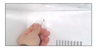
1) Remove screw cap on the Freezer Louver.
