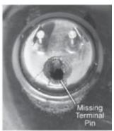
FIGURE 1-3: Close up view of hermetic teminal after it has vented.
