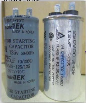
Running Capacitor 250VAC-12 \mu F Starting Capacitor 125VAC-125 \mu F
