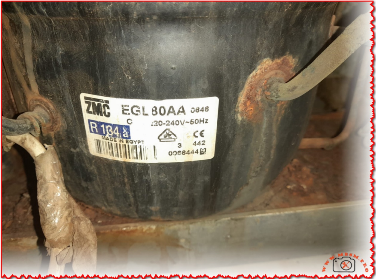
Mbsm.pro, Compressor, ZMC, coolant R134a, 150 G, EGL80AA, GL80AA, 220-240V 50Hz, fully hermetic, 9kg, 1/5 HP, power input 162W, EGYPTIAN CO. FOR INDUSTRIALIZATION, FB30, 280L
