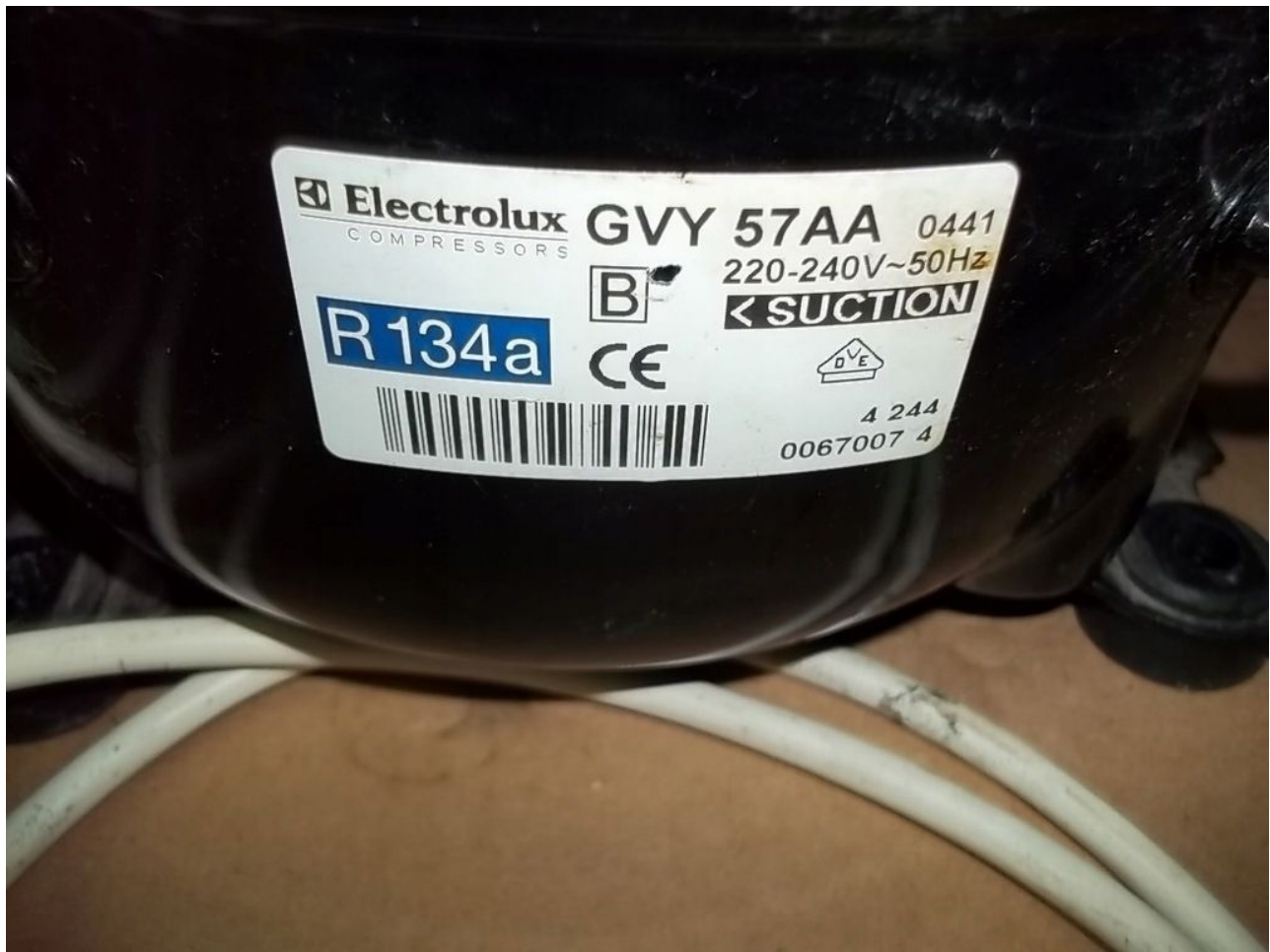
Mbsm.pro, Compressor, ZEL, GUY57AA, 1/5 hp, Acc, r134a
