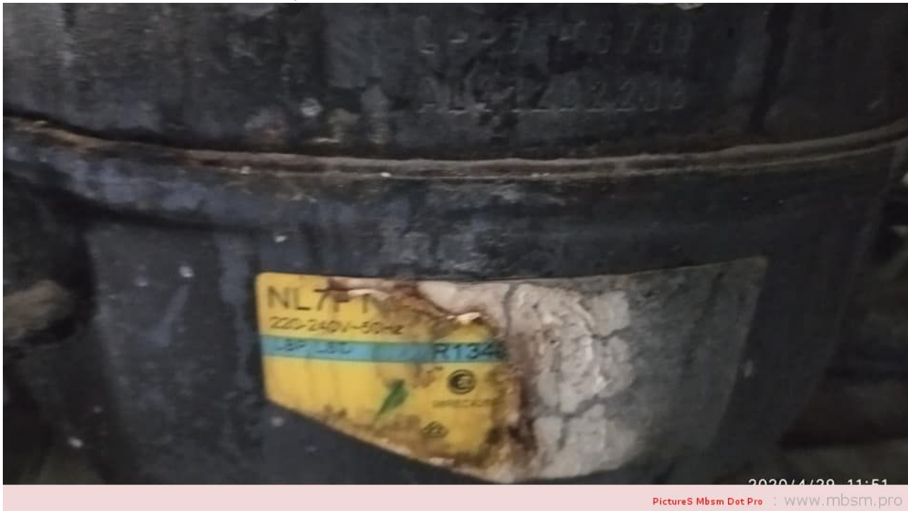
Danfoss ,Fridge Compressor ,NL7FT , 1/4 HP ,R134a
