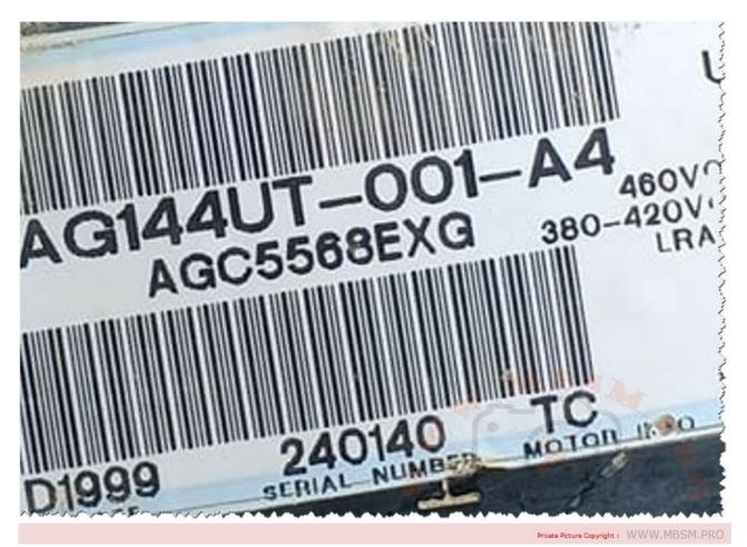
Mbsm.pro, Compressor , Air Conditioning, r22, Tecumseh, AGC5568EXG, AG144UT-001-J7, 5-1/2 HP, 4 ton, R-22, 56700 btu, HBP/AC
