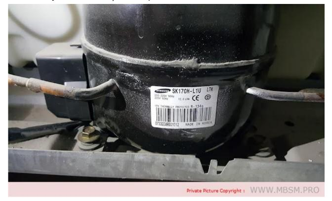
Mbsm.pro, Samsung, SR-40RMB, Refrigerator, compressor, sk170h-llu, 1/4 hp, r134, lbp, 195 w
