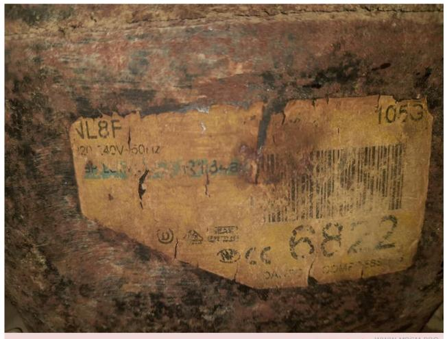
Mbsm.pro, Compressor, SECOP, NL8F, R134A, 1/4 hp++, 1/3 hp-, 105g 6822, 105g6822
