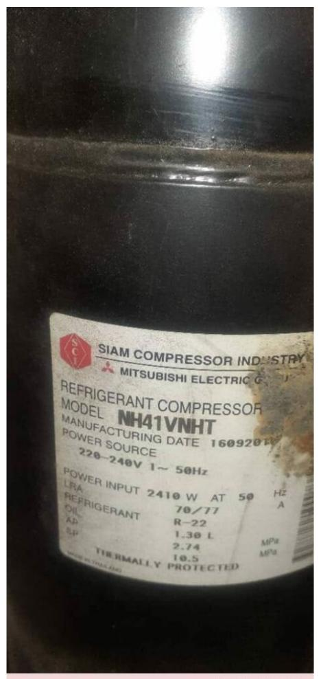
Mitsubishi, Electric, fixed frequency, NH41VNHT 2.55HP, single-phase, 220V, rotary, air condition, 26000 btu/h
