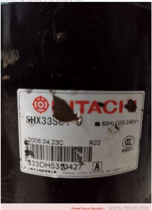
Mbsm.pro, compressor, Highly, hitachi, rotary, SHX33 , 2 hp, 17750 btu, R22
