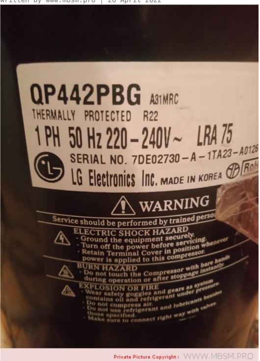
Mbsm.pro, Compressor Lg, 26000 btu/h, QP442PBA, LG, AC Rotary Compressor, Rotary Scroll Compressor, 220-240V 50HZ, 2 ton, 3 Hp, 1 PH
