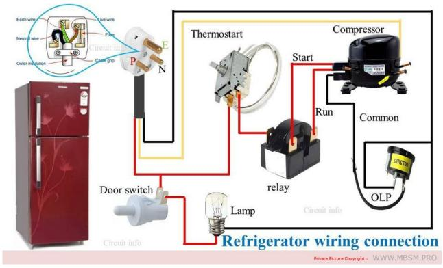
Mbsm.pro, PIctures, refrigerator wiring connection
