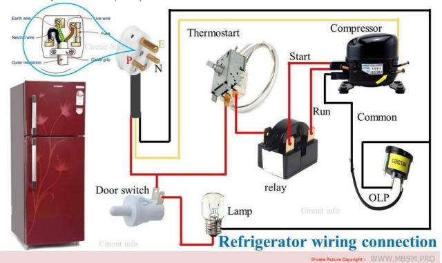
Mbsm.pro, PIctures, refrigerator wiring connection
