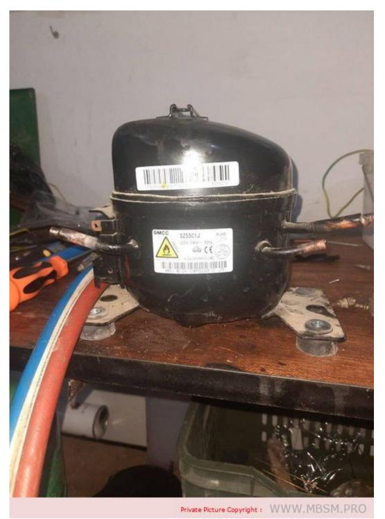
Mbsm.pro, Refrigerator, Mini compressor, GMCC, C Series, TOSHIBA, SZ55C1J, HRD-071S, 75 w, 1/10 hp, LBP, r600a
