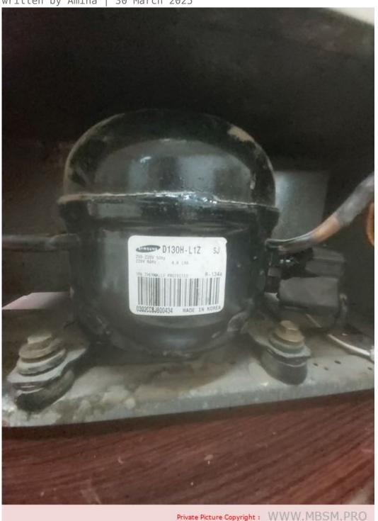
Refrigeration, Compressor, 1/10 HP, R-134A, Samsung, CD130C-L1Z2
