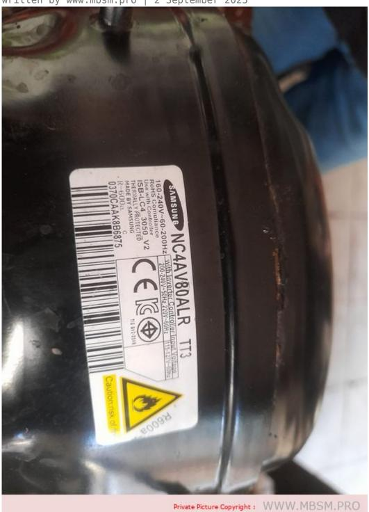
Mbsm.pro, Compressor, Samsung, Nc4av80alr, 1/4 hp, Displacement 8.08cc, Inverter, type Nc, R600a, Lbp, serie AV, Blcd Control 9 slot
