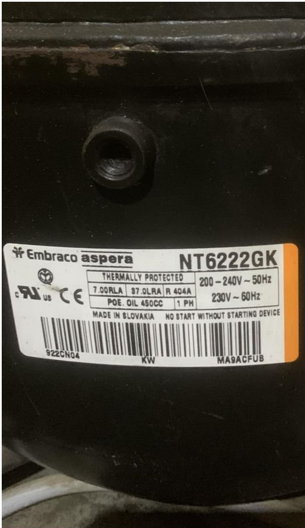
Mbsm.pro, Aspera, Embraco, NT6222GK, R404A, R449A, R407A, R452A, 3/4 hp++, MHbp, 1 Hp-, Dis 17.39 cm 3
