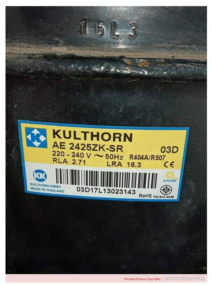
Kulthorn, Kirby, Compressor, AE2425ZK, ae 2425zk-sr, R404, 1/2HP, Hermetic piston compressor, AE2425ZK-SR, Application: low temperature, Displacement: 14.14 cm3, Cooling capacity: 613 W, 220 V / 50 Hz / 1 phase.
