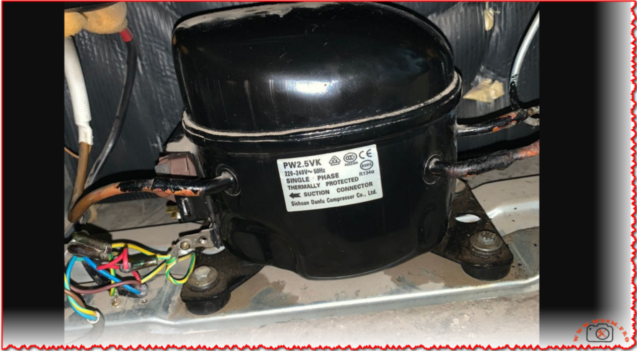
Mbsm.pro, Pw2.5vk, 1/12 hp, Refrigeration, Compressor, R134a, 220~240v Ac 50hz, Mbp/lbp, Sichuan Danfu Compressor
