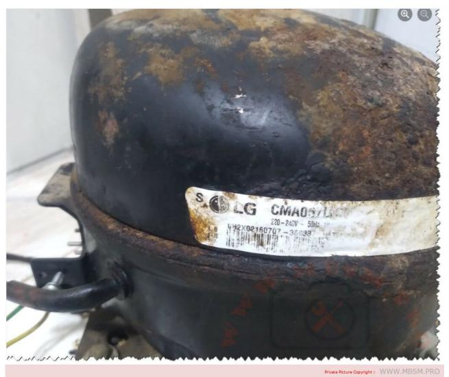
Mbsm.pro, LG, CMA057LHEG, 1/5 hp, R134A, 135 g, Alu Wire, compressor, lbp, 160 w, 1ph, BCD-192, SWAIDY, REFRIGERATOR
