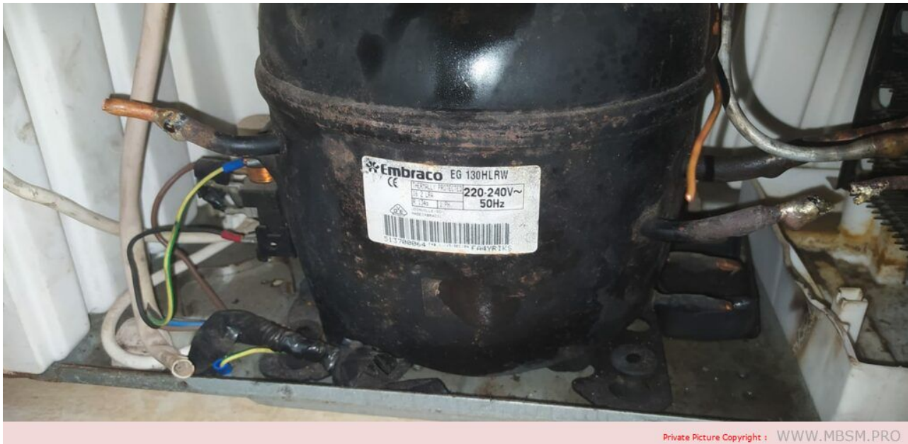
Mbsm.pro, Compressor, EMBRACO, EG130HLRW, r134a, 1/3 hp, LBP, RSIR-CSIR
