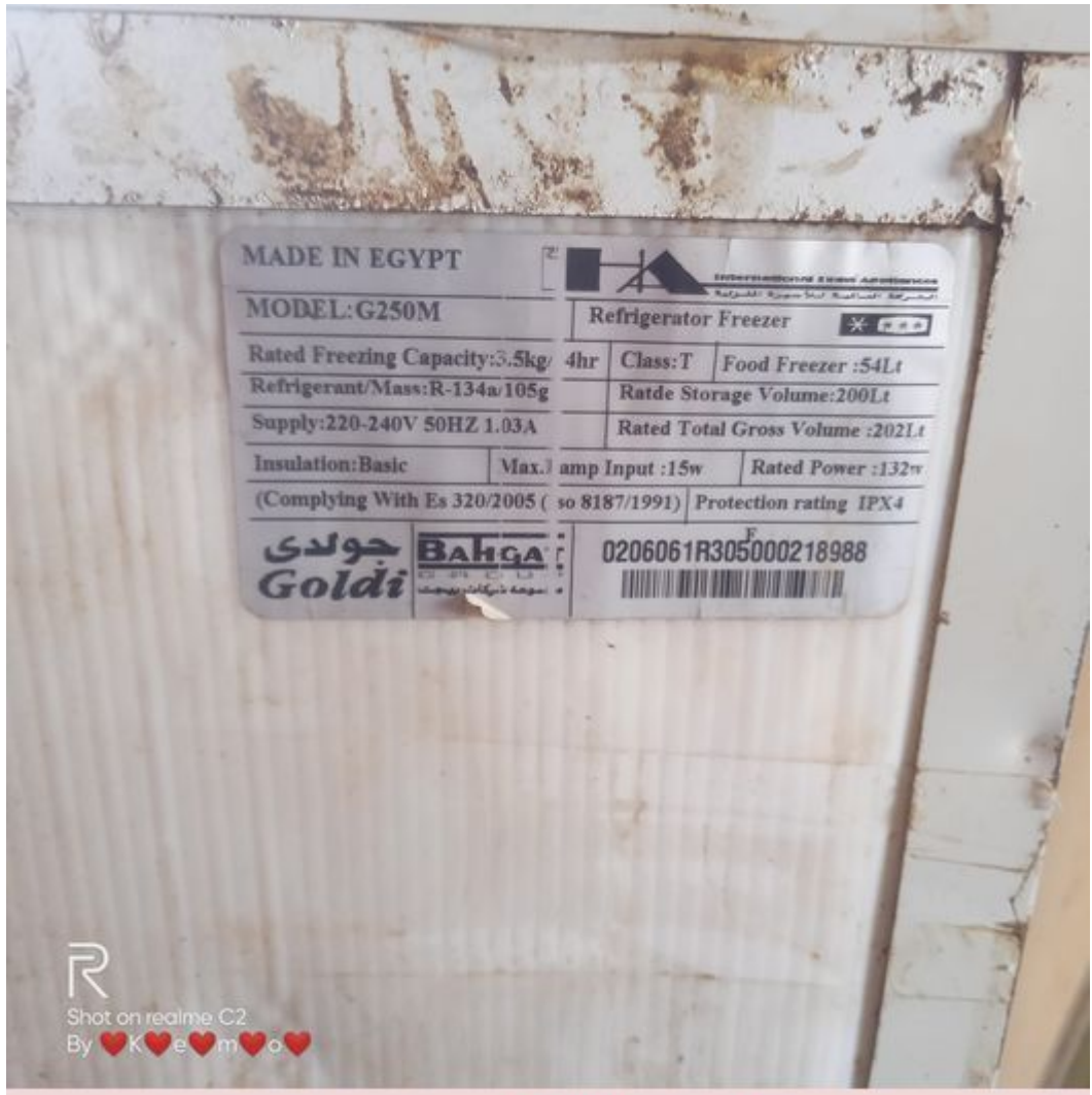
Mbsm.pro, refrigerator, Goldi, G250M, 250 L, 9 feet, compressor, 1/8 hp, r134a, 105 g, classe T
