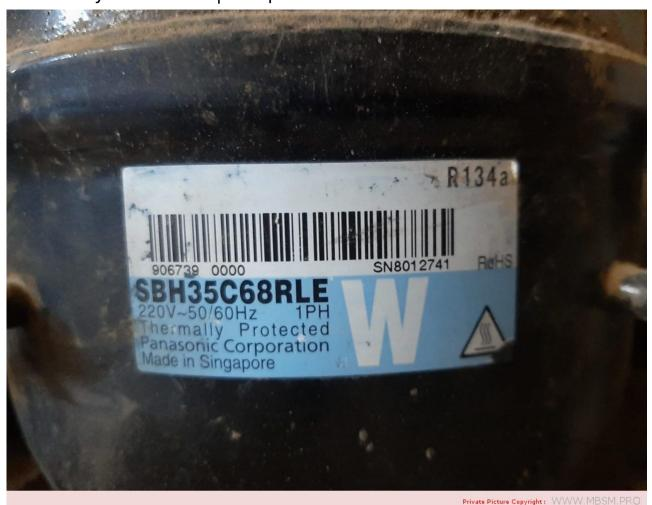
Mbsm.pro, Compassor, Panasonic, SBH35C68RLE, 1/8 hp, 100 w, 3.5cm<sup>3</sup>, 220 v 50hz, R134a, Refrigerator, freezer, Sharp,
