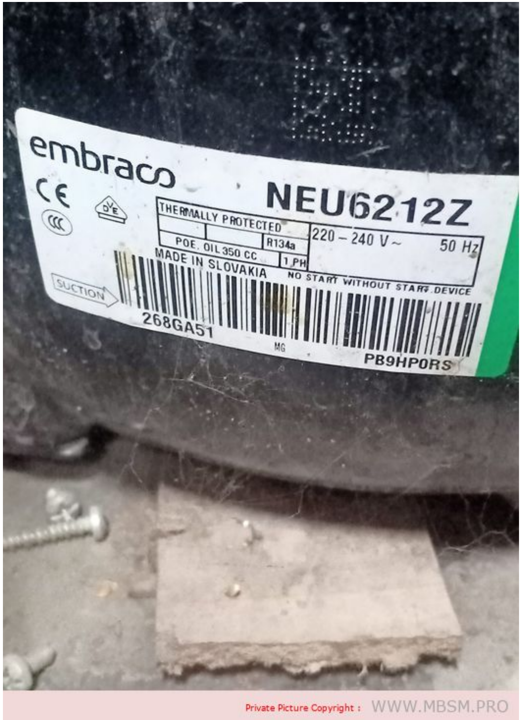
Mbsm.pro, Compressor, NEU6212Z, 1/2 hp, EMBRACO, ASPERA, R134A, hbp
