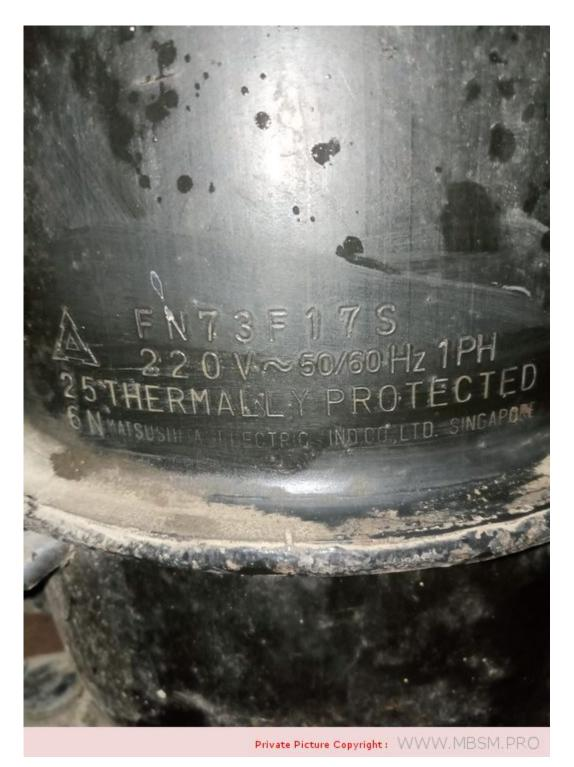
Mbsm.pro, FN Series, Commercial, Refrigerator, Compressor, R134A, fn73f17S, 1/5 hp, FN75H, 1/6HP, FN77H, 1/4 hp, R12, LBP, 220V-50/60HZ
