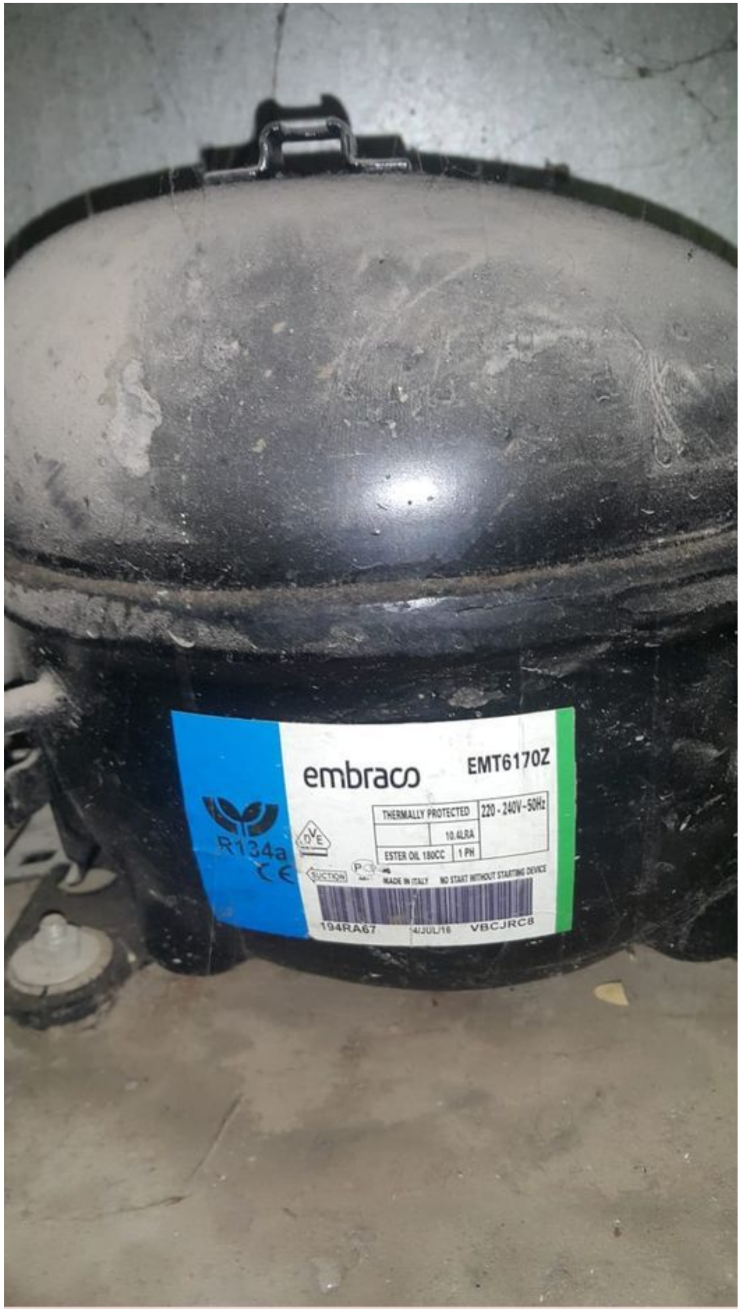
Mbsm.pro, Compressor, EMBRACO, EMT6170Z, HBP, R134a, 350 G, 220-240V/1F/50Hz,
