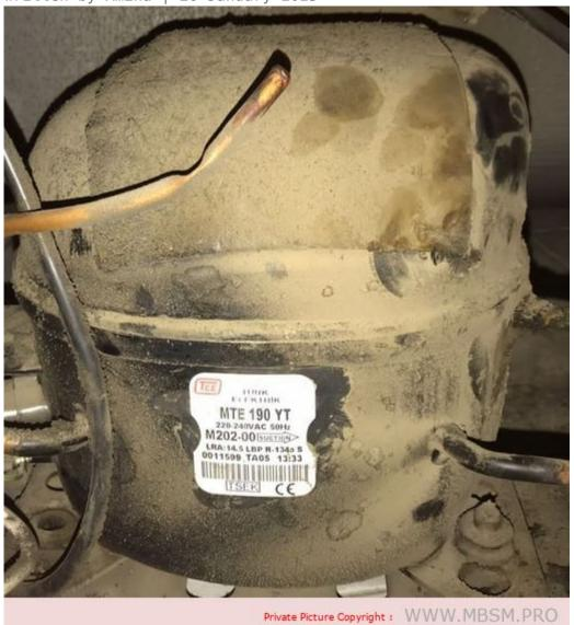
Compressor, Tee, Turk, mtel90yt, 1/4 hp, Double door refrigerator, r134, Lbp, 189 W
