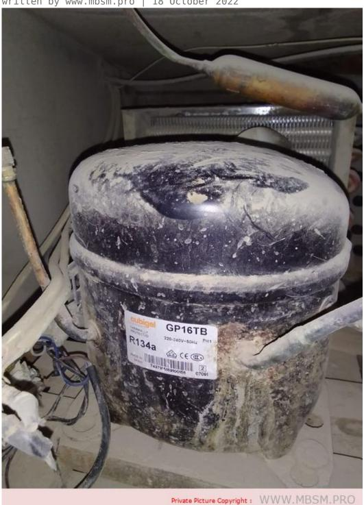
Mbsm.pro, Cubigel, GP16TB, hermetic, compressor, 3/8 hp++, 1/2 hp-, HBP, R134a, R1234yf, CSIR,
