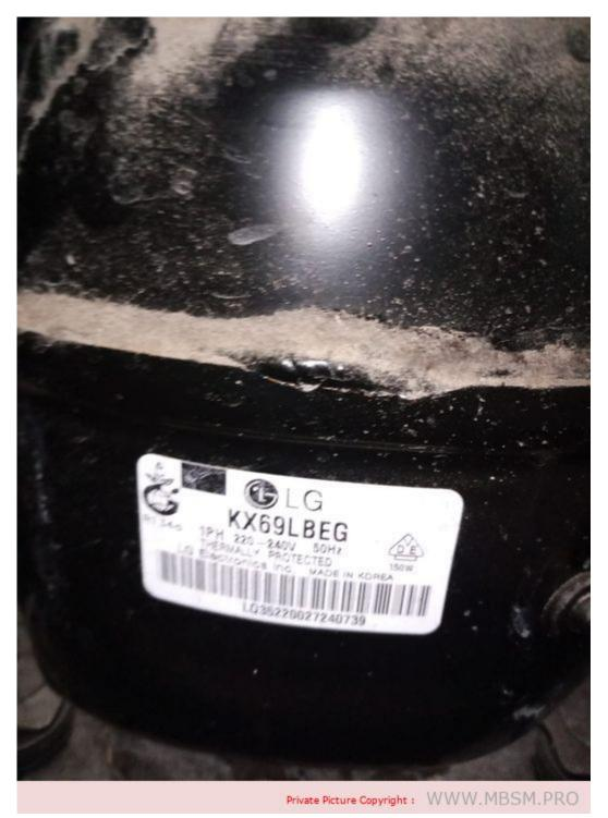
Mbsm.pro, Compressor, kx69Lbeg, LG, Serie Kx, 1/5 hp++, 1/4 hp-, Lbp, r134a, 220-240v, RSIR, PTC, 190 w, capillary 0.040
