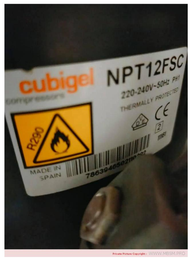
Compressor, NPT12FSC, CUBIGEL, R290, 12,10ccm, LBP, 3/8HP, 220 V 50/60 Hz
