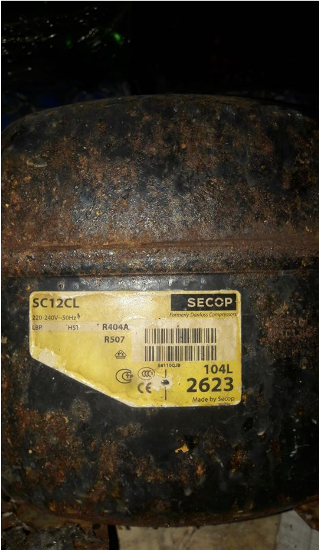
Compressor Danfoss SC12CL 3/8 HP , LBP/MBP, R404A/R507
