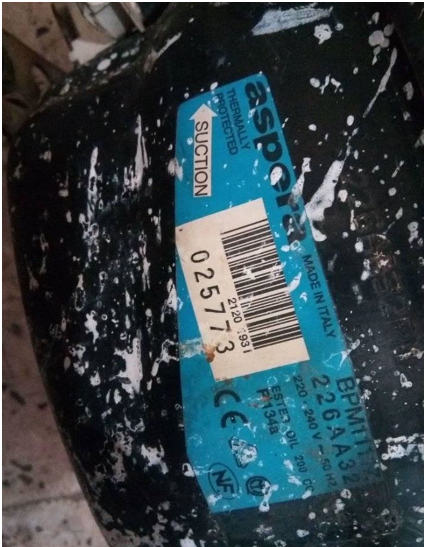
Compressor Bpm111z , r134a 1/6hp ,5.6cc, 240v 50hz ,ASPERA, EMBRACO
