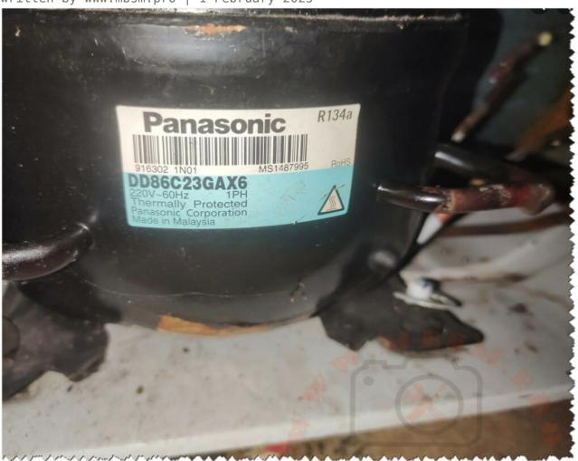
Mbsm.pro, Panasonic, Compressor, D Series, DD86C23GAX6, 1/3 hp, 300 w, lbp, r134a, 8.6 cm<sup>3</sup>
