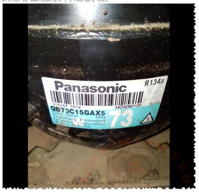
Mbsm.pro, Freezer, GR-EF40, TOSHIBA REFRIGERATOR-FREEZER, 335 L, Qb73c15gax5,R134a , Refrigeration Compressor ,1/4 Hp, Panasonic, QB series , 1Ph , 220V 50Hz
