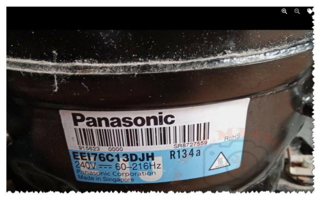
Mbsm.pro, Compressor, EE 76613DJH, Panasonic, inverter, Blcd, 1/5 hp, from to 50 to 260 hz, lbp, r134a, EEI Series
