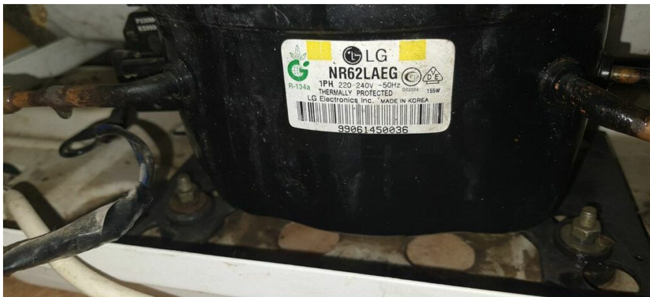
Mbsm.pro, compressor, Lg, Nr 62 LAEG, Nr62LAEG, r-134, 1/5 hp
