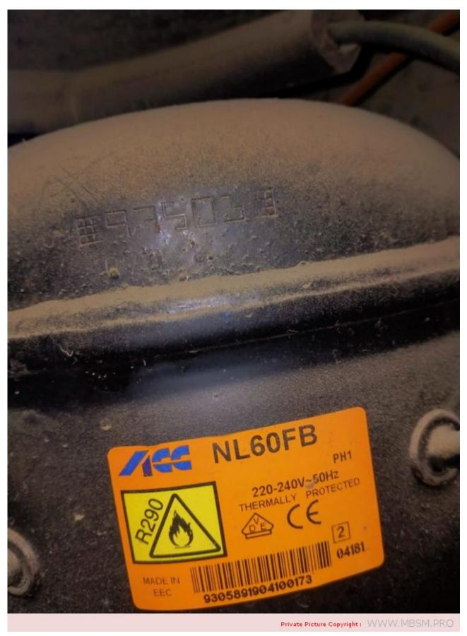
Mbsm.pro, Compressor, NL60FB, 1/5 Hp, Lbp, R290, 220v, 1 phase 50 hz
