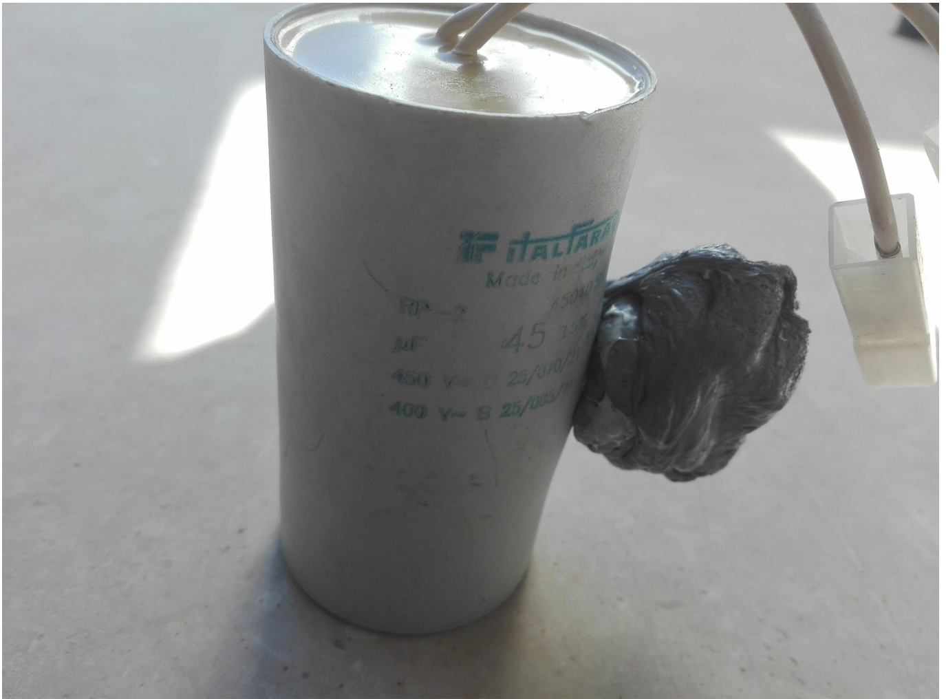
mbsm-dot-pro-capacitor-explodes- Pictures-F.jpg (748 KB)
