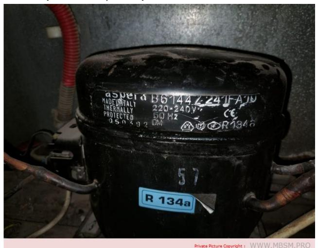
Mbsm.pro, Compressor, NB series, NB6144Z, AE8LMY, B6144Z, 1/5 hp++, MED/HIGH, 1/4 hp-, Emkarate RL22HB POE lubricant,
