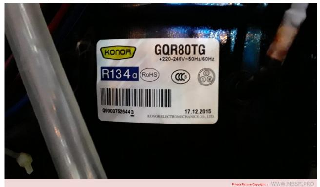
Mbsm.pro, Compressor, SIKELAN, GQR80TG, 1/4 hp++, HBP, 1/3 hp-, Refrigeration, R134a, 220-240V 50HZ, MQ-GQR80TG, GQR80TG
