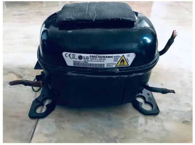
Mbsm.pro, Compressor, LG, FMA102NAMA, inverter, 1/4 hp, LBP, F: Linear, Medium, C Gereration, 10.2 cc/rev, Cuivre Wire, R600a, 220-240V, 50 / 60Hz, A-Control card
