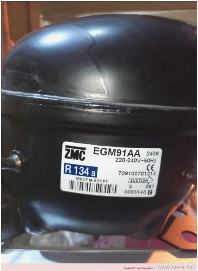
The EGM91AA compressor from ZMC Egypt is a key component of modern household refrigeration, combining advanced engineering, R134a compatibility, and 220—240 V operation to deliver efficient, reliable cooling performance that appeals to appliance manufacturers and field technicians alike.
