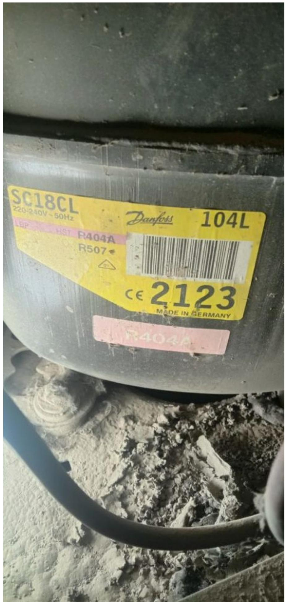
Mbsm.pro, Secop, Freezer, Compressor, Sc18cl, 104L2123, 5/8HP++, 1/2-, R404A, Secop SCxxCL Series, LMBP, 495 w
