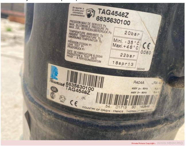
Mbsm.pro, Compressor, Tag4546X, Tag 4546X, Tecumseh, 400 v / 3 Ph, 4 Hp, 34000 btu/h, 8500 kcal/h
