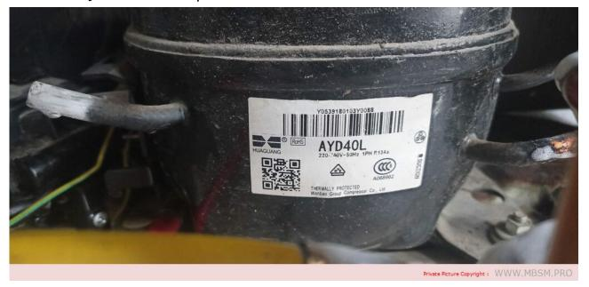
Mbsm.pro, Huaguang, ayd40l, R134A, 220V/50Hz, 1/8HP, 108W, refrigerator, compressor, Wanbao Group Compressor
