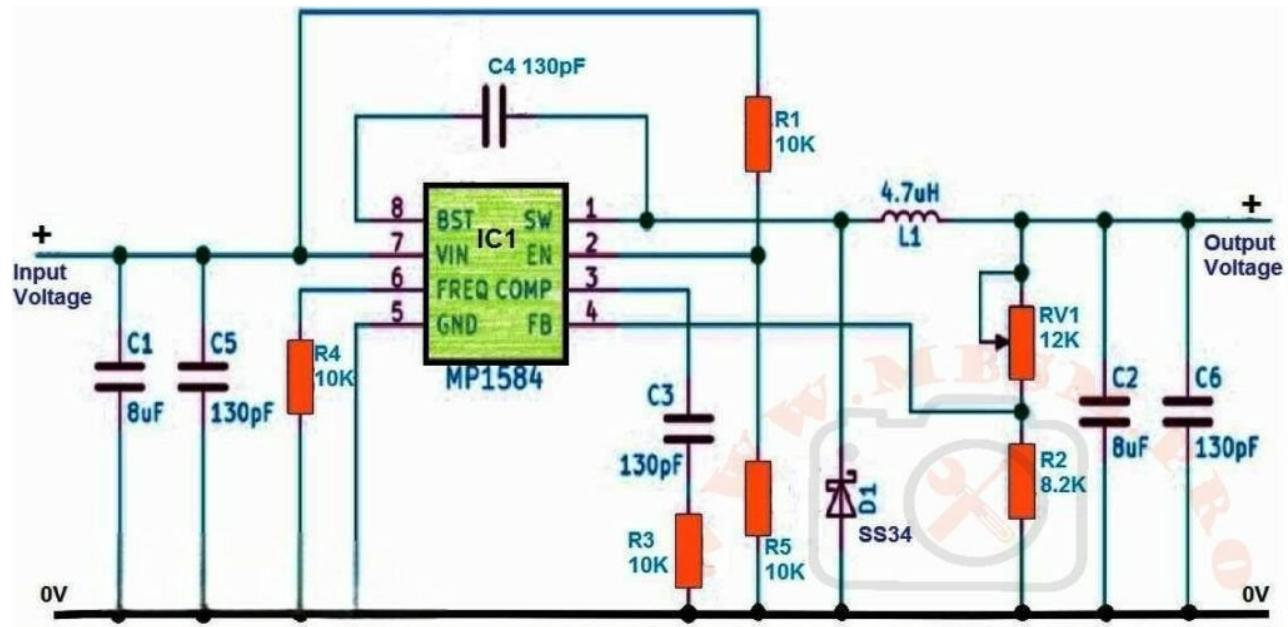
Mbsm.pro, 3A Adjustable voltage regulator circuit from 12 v to 5 v DC
