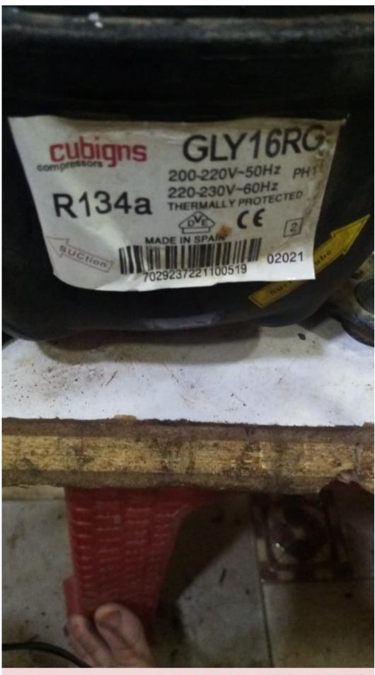
Commercial refrigerator, compressors, GLY16RG, 3/8 hp++, R134a, HMBP, 1492W, r134, Compressor ACC, Cubigel, Huayi, Electrolux, ZEM
