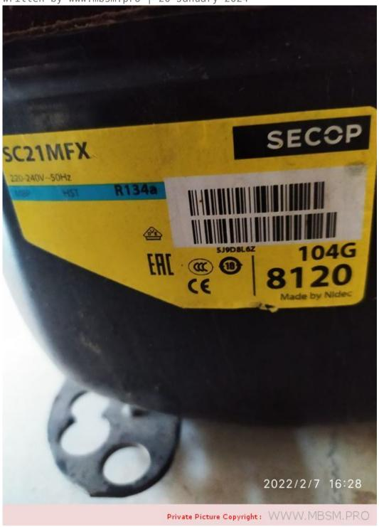
Mbsm.pro, Compressor, Danfoss, Secop, 5/8 hp++, SC21MFX, MBP, R134a, 220 V-240
