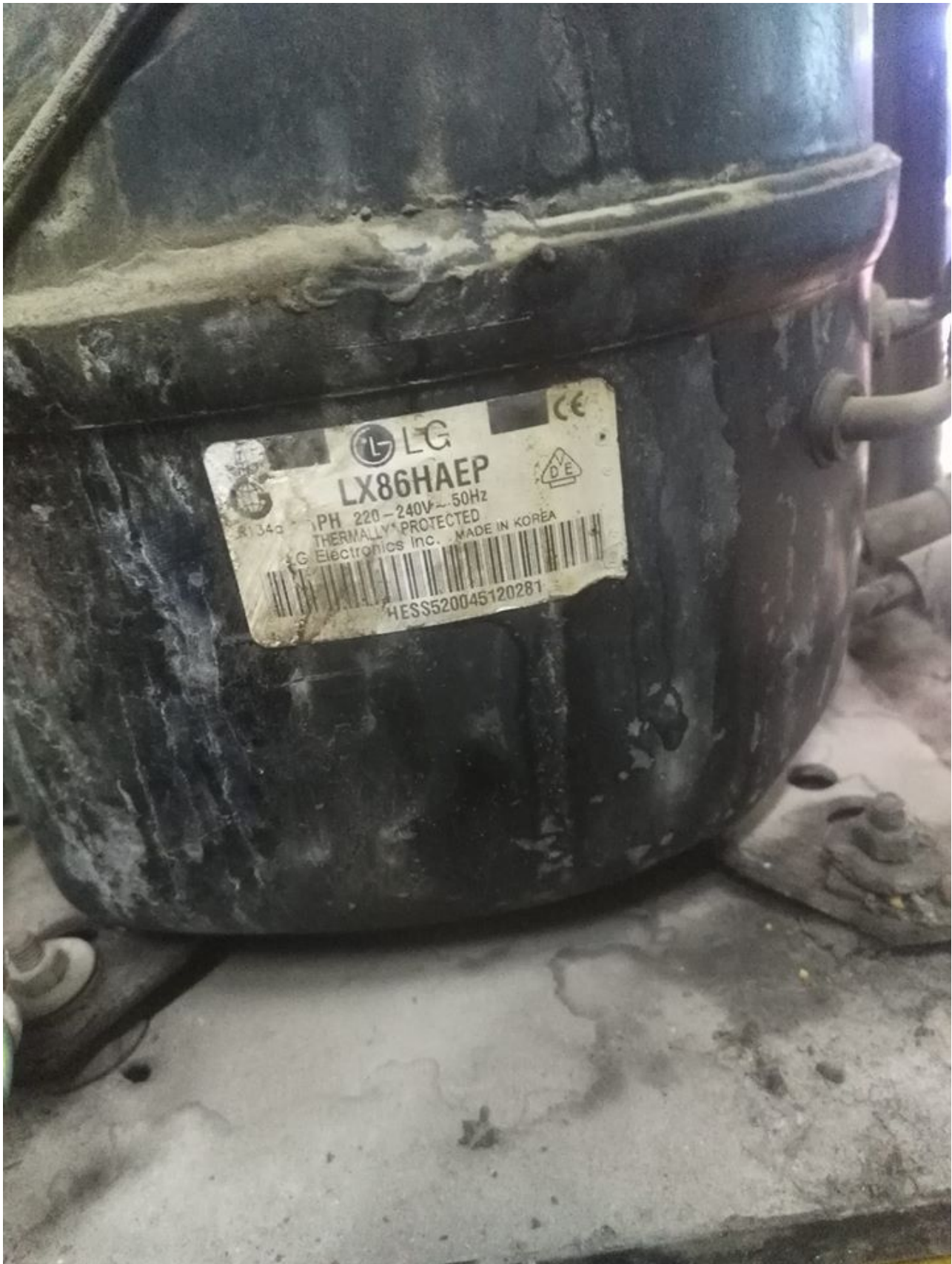
LG Refrigeration Compressor ,LX86HAEP , 385 w , 220 v 50Hz , R134A ,1/2 Hp
