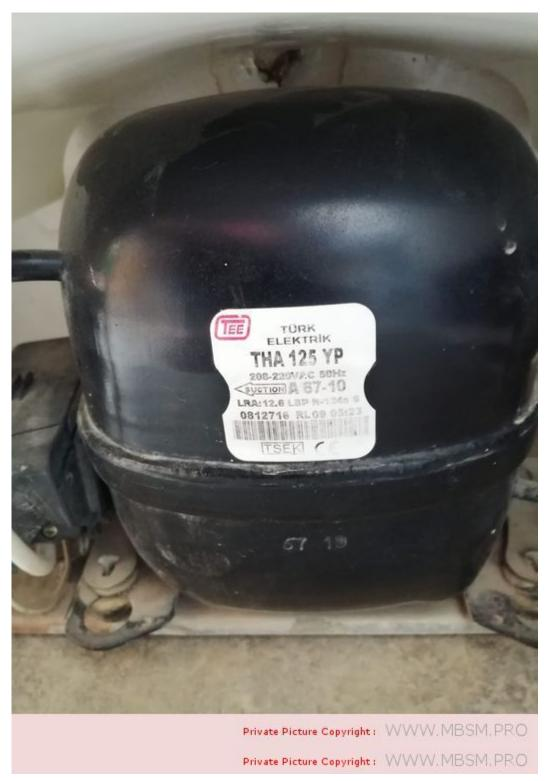
Mbsm.pro, Compressor, THA125YP, 1/5 Hp, 145 W, Tee compressor, 125 Kcal/c, R134A, Lra 12.6 A, 208-220 vac 50 hz
