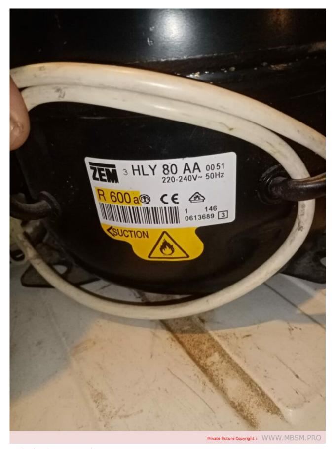
Technical Data Sheet Compressor model HLY80AAa Voltage 220-240V 50Hz ~1 Refrigerant R600a
