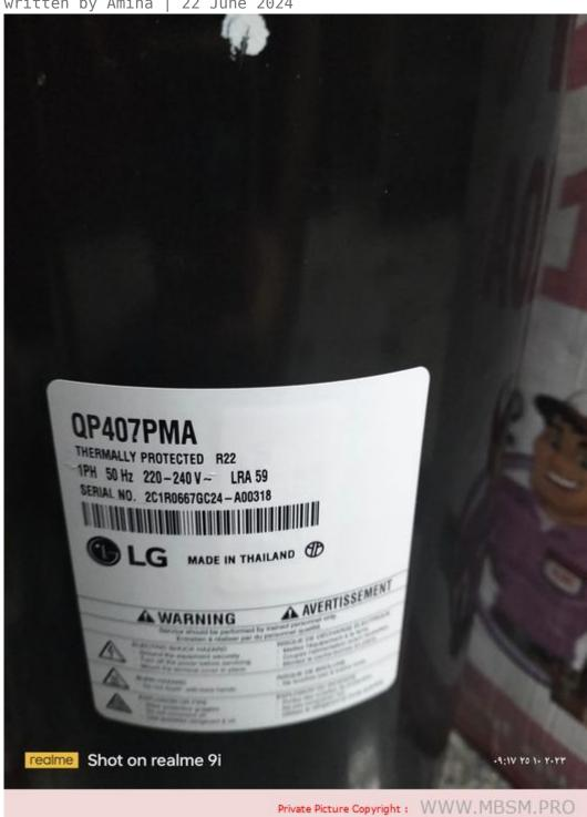
Compressor, LG, QP407PMA, 2.5 hp, r22, 24045 btu, 7048 w
