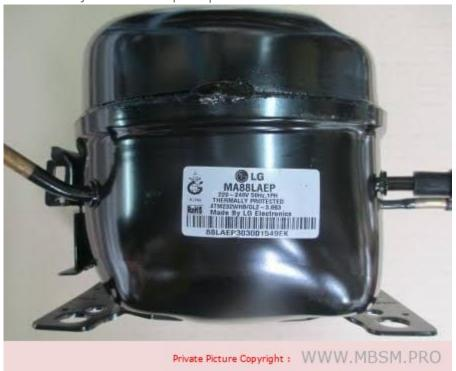
Mbsm.pro, LG, MA88LJJP, 1/3 hp, Refrigerator, Compressor, (410-450 litre), lbp, 235 (kcal/h), 273W, 933 (Btu/h), 0.367HP, input power 220w
