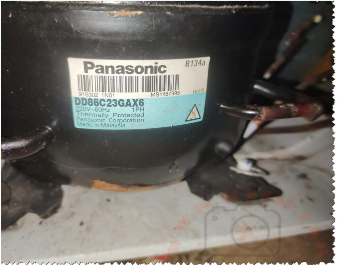
Mbsm.pro, Panasonic, Compressor, D Series, DD86C23GAX6, 1/3 hp, 300 w, lbp, r134a, 8.6 cm 3
