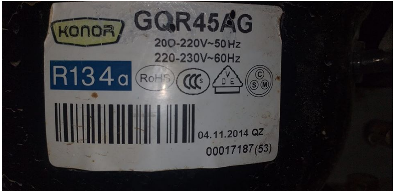
1/8hp refrigeration compressor, R134a, KONOR ZANUSSI, GQR45AG, LBP, RSIR
