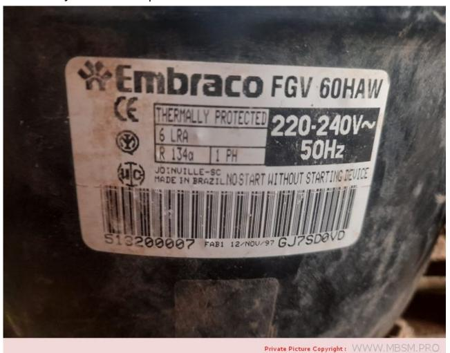
Mbsm.pro, Compressor, FGV60HAW, EMBRACO, 1/5 hp, r134a, 220-240V 50Hz, lbp, 147 w, 500 btu
